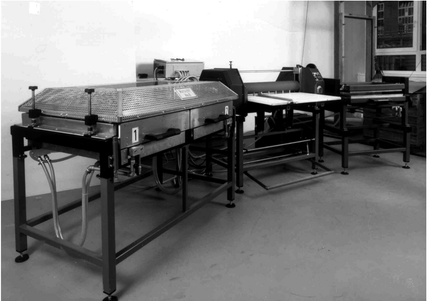
Figure 32: Equipment for heat lamination: heating station, rolling unit, cooling jig (from left to right)
